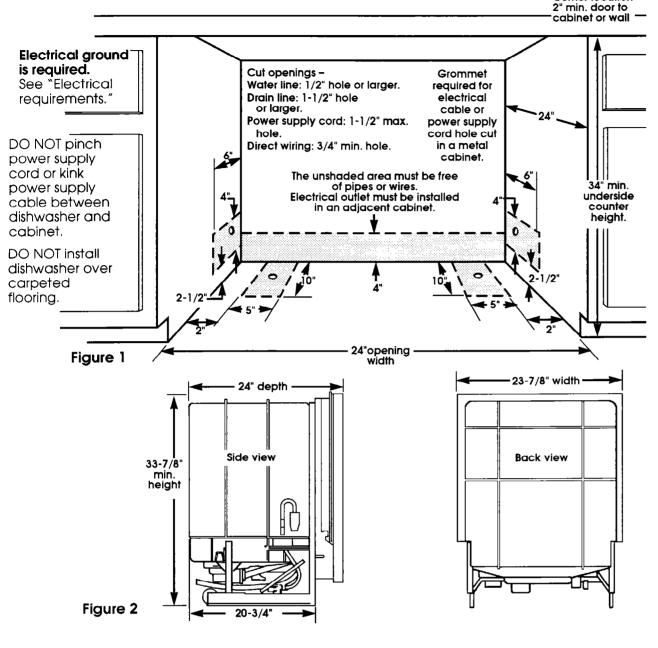
Check location where dishwasher will be installed. The location should provide:
